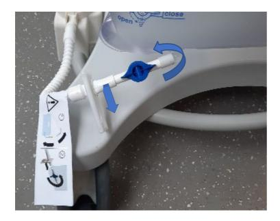
➤ Open the occlusion clamp and drain valve. Pump head automatically fills with fluid.
