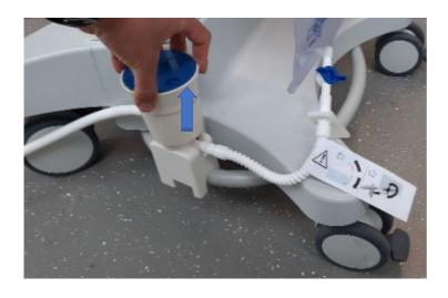
> Remove the pump drive by pulling it vertically upwards.
