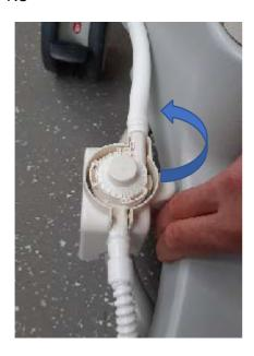
➤ For the multiFiltratePRO device, hold the housing with slight pressure and remove the holder with the pump head in the direction of the arrow.
