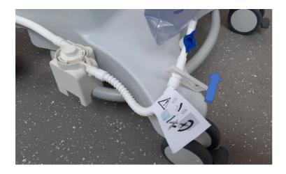
Connect the drain line (short tubing) to the filtrate bag outlet.
